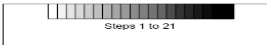
Figure 4 Representation of a Sensitometry Strip with 21-Steps of Measured Densities
